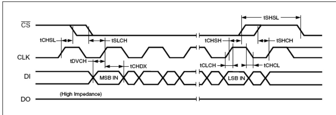
**Figure 24. Input Timing**
