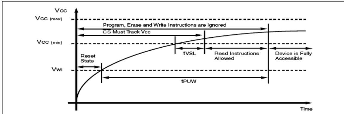
**Figure 21. Power-up Timing**
