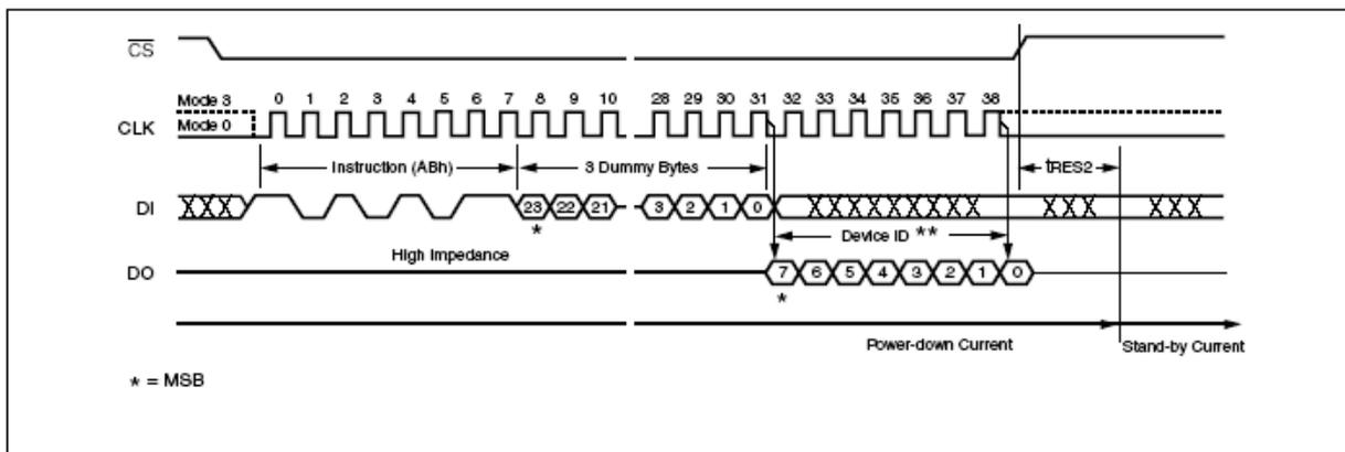
**Figure 17. Release Power-down / Device ID Instruction Sequence Diagram**
