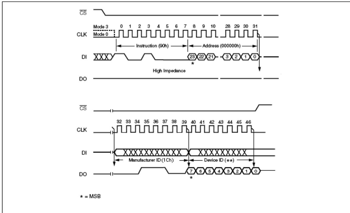
**Figure 18. Read Manufacturer / Device ID Diagram**
